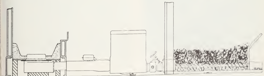
25-2. A cross sectional view of a stoker installed in a furnace and a coal bin. (Iron Fireman Mfg. Co.)
